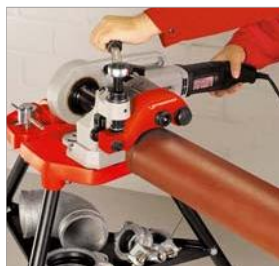
Use with roll grooving tool ROGROOVER
