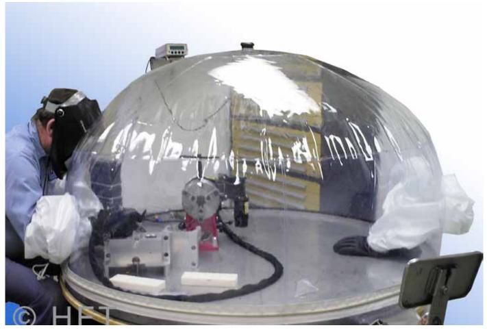
The **Argweld®** range of **Flexible Welding Enclosures™** has been designed for applications where a rigid chamber may not be economically viable or where space may be at a premium.
